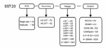
For example: if order a dual-axis SST20 inclinometer, range  $\pm 60^{\circ}$ .  $\pm 0.07^{\circ}$ accuracy, output CAN2.0B, the model should be chosen as : SST20-02-P2-60-G3
